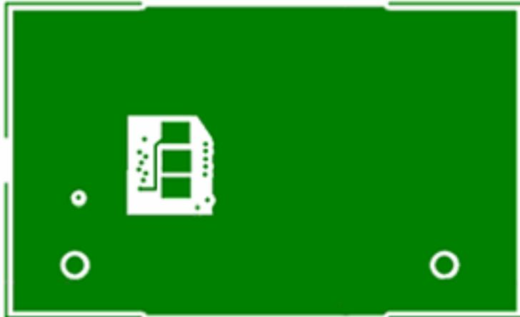
Figure 17. SP7662EB PC Layout 2<sup>nd</sup> Layer Side
